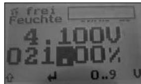
5. To save the values you have to leave the “Moisture” menu item by pressing the shift button ( ⬆ ) first, and then the symbol with the opened door ( ⬆ ).
